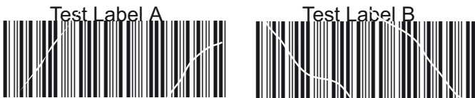
Possible printouts due to ribbon wrinkling
